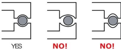
Over tightening the saddle rail clamp could cause breakage of the rails, and be the cause of accidents. Always consult the owner's manual of the mating seatpost. If the seatpost's torque recommendation exceeds the saddle's recommendation always use the lower torque.
