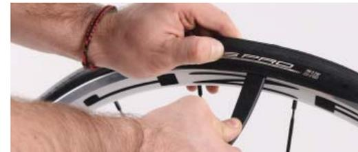
5. Make sure the inner tube is not trapped between the rim and the tire (see fig.5), and that the valve is perpendicular to the rim (see fig.6). Inflate the tire slightly (1 bar/15 psi) and verify the correct positioning of the valve by pressing it gently upwards. Spin the wheel and check the perfect alignment of the clincher and the correct fit of the tire bead.
